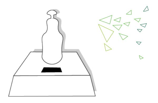
When we're start to use the sanitizer, we can easily put our hands under the dispenser WITHOUT touching and then it will automatically pour the liquid down. It will stop once we place our hand far from the sensor. In this prototype, I am designing the house for the hand sanitizer dispenser along with all of its components.
